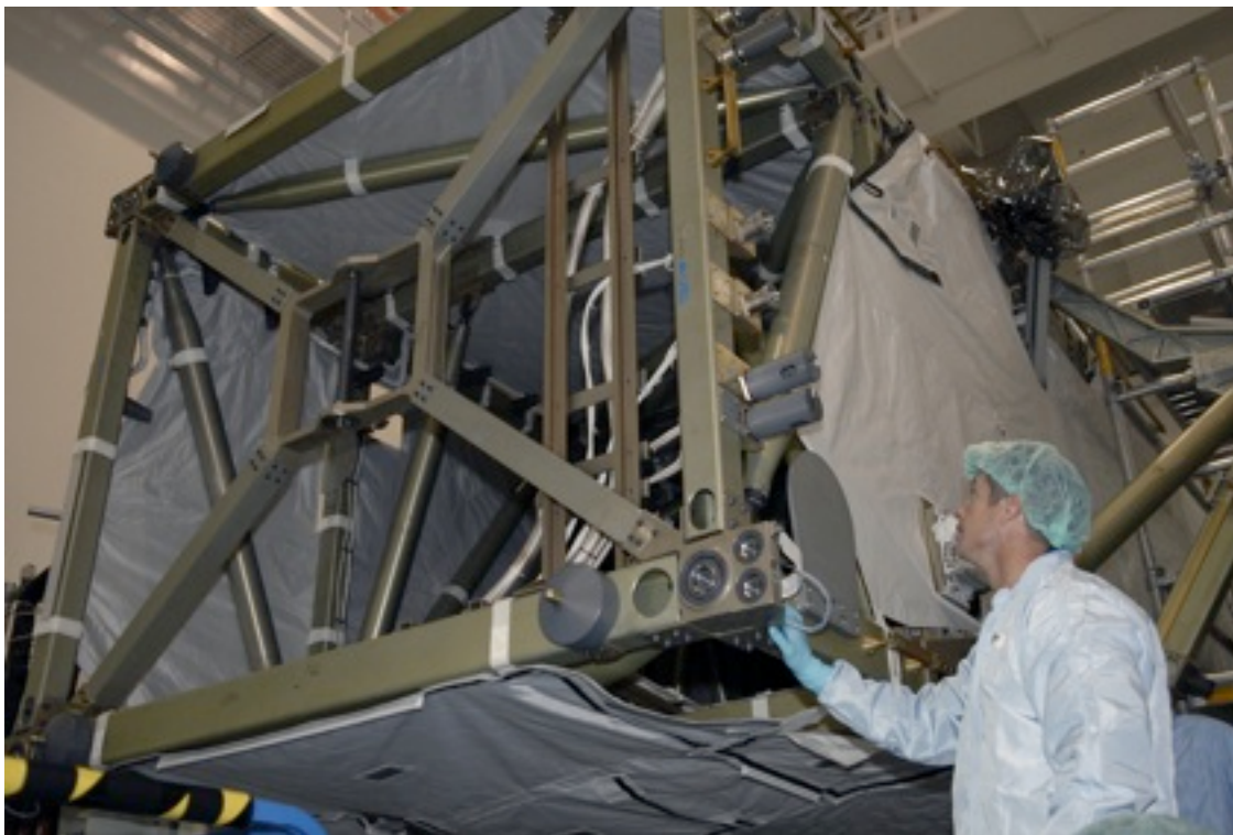
Astronaut Steve Swanson inspects the attachment fittings that will hold the S6 solar array truss segment in place on the right end of the space station's power truss.
