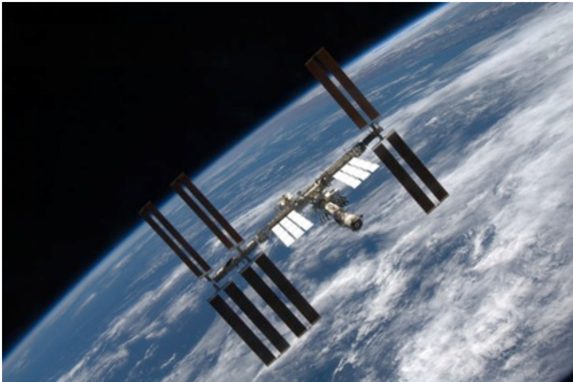
The International Space Station in its current configuration. The P4 and P6 solar arrays are visible on the left side of the station's main power truss while the S4 segment stands alone on the right side. The new S6 truss segment will be attached to the right side during Discovery's mission
