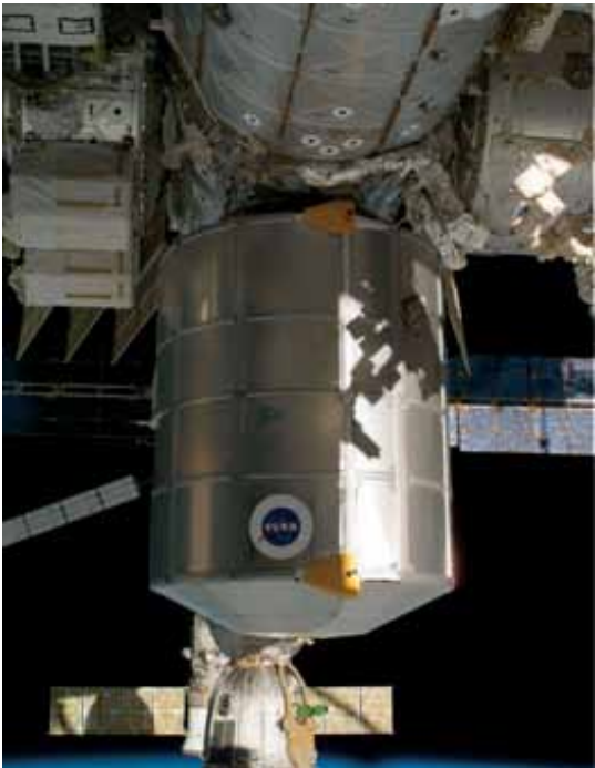
The Permanent Multipurpose Module (PMM) is shown shortly after being attached to the Unity module during space shuttle mission STS-133.
