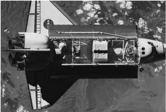
Space shuttle Endeavour approaches the ISS during mission STS-118 with the S5 truss section ready to be installed
