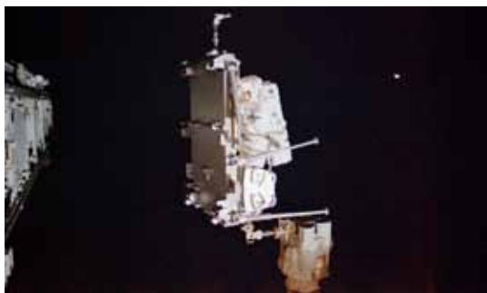
Mission specialist John Herrington, anchored on Canadarm2, moves the CETA during an STS-113/ISS-11A EVA.
