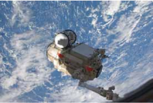
In the grasp of Canadarm2, MRM1 is transferred from Atlantis's payload bay to be attached to Zarya on the ISS.
