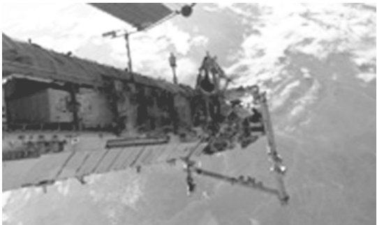
P3/P4 truss being installed during space shuttle mission STS-115/ISS-12A
