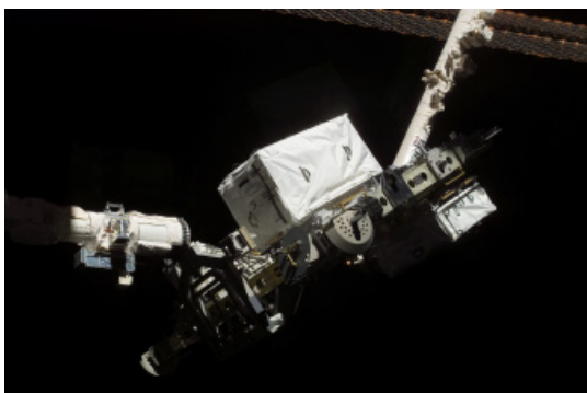
The space shuttle robotic arm moves away following the hand-off of ESP-3 to the station's robotic arm while docked with the ISS during mission STS-118/ISS-13A.1.
