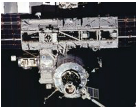
Central integrated truss (S0) following installation during space shuttle mission STS-110/ISS-8A
