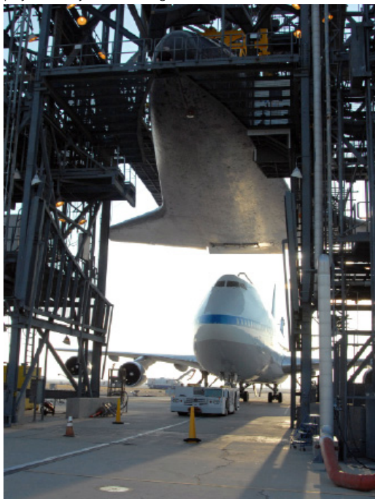
At EAFB, the SCA is towed beneath the orbiter, suspended in the MDD.
