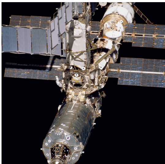
The Destiny Laboratory after its delivery and installation by the STS-98/ISS-5A crew, as seen from the departing space shuttle Atlantis
